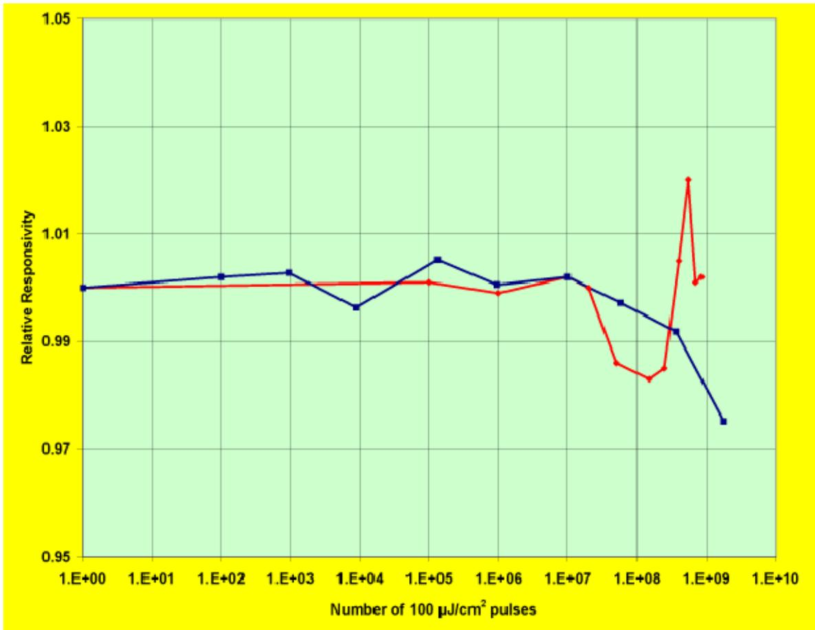
**Fig. 2:** Responsivity stability of SXUV series photodiodes after exposure to 193 and 157nm excimer laser:
