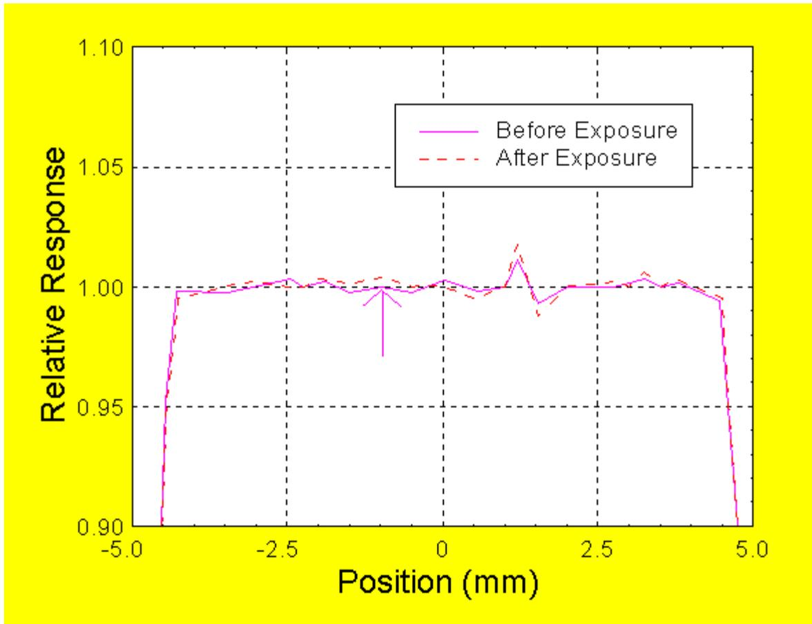
**Fig. 4:** Line scan of the SXUV-100 diode with 12.4 nm beam before and after exposure to  $10^{22}$  photons/cm<sup>2</sup> 100 eV photons
