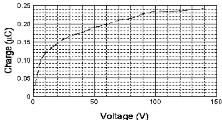
**Fig. 1:** Charge seen by external circuit as a function of photodiode bias for UVG-20. 193 nm
